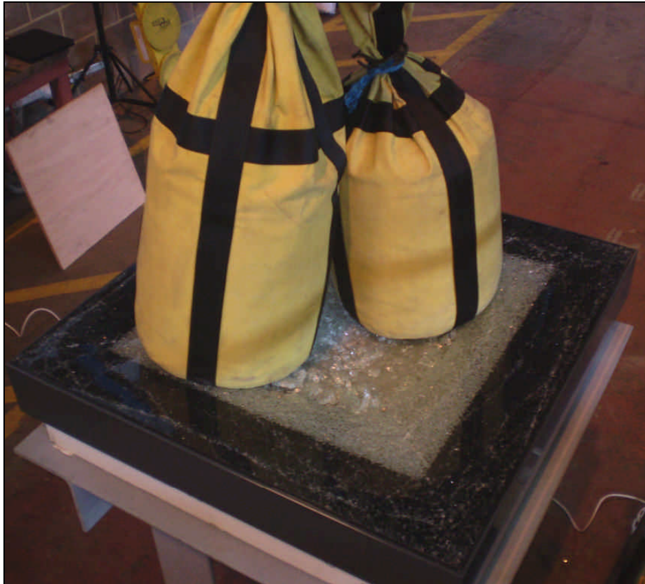
SAMPLE 1 WITH 90 KG STATIC LOAD
