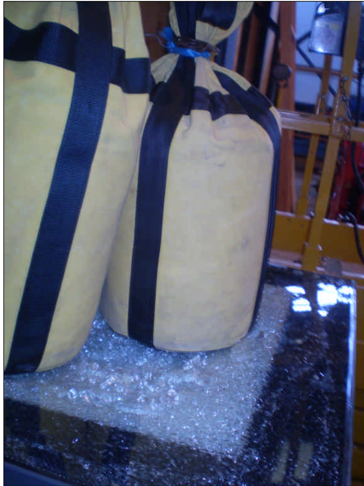
SAMPLE 2 WITH 90 KG STATIC LOAD
